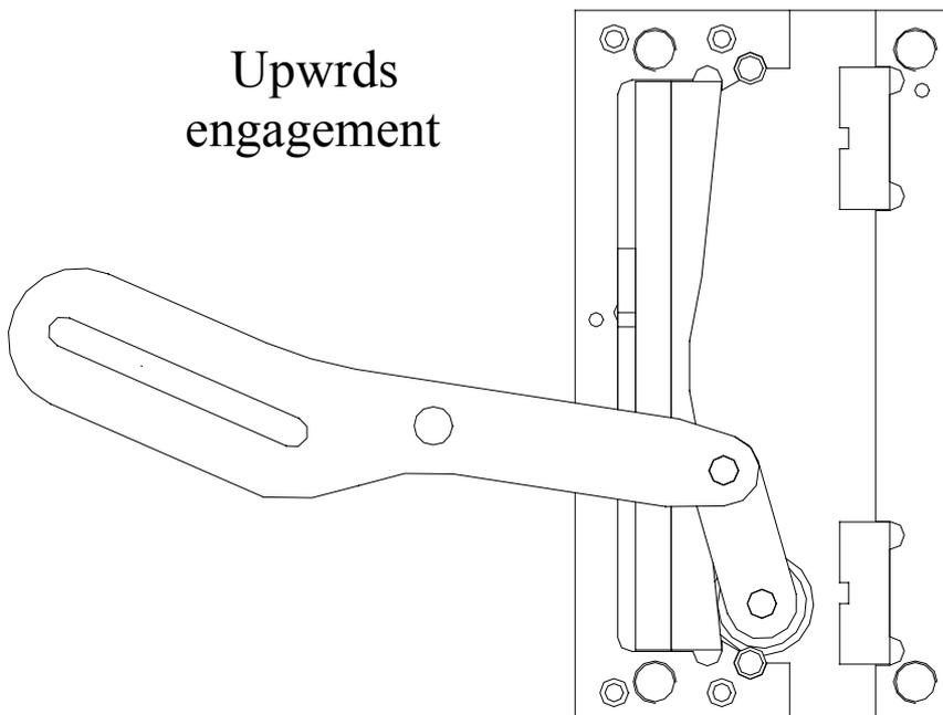
As a suggestion for the safety gear fixing to the sling, the tightening torque of 8.8 M12 screws is 79.09 Nm and 111 Nm for those of 10.9.
